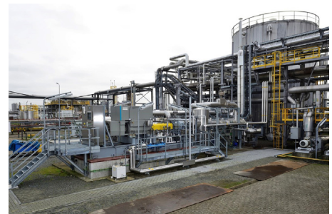
Left picture: Integrally-g geared refrigerant compressor (using a natural refrigerant). Right picture: A heat pump / mechanical vapor compressor with direct steam compression cycle applied in a chemical plant.
