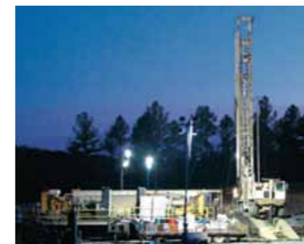
The RD20 is a high production rig with capability to drill wells to depths in excess of 5,000 ft.
