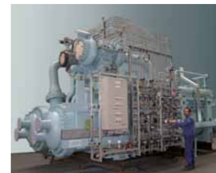
A Comander for on-board reliquefaction of LNG.
