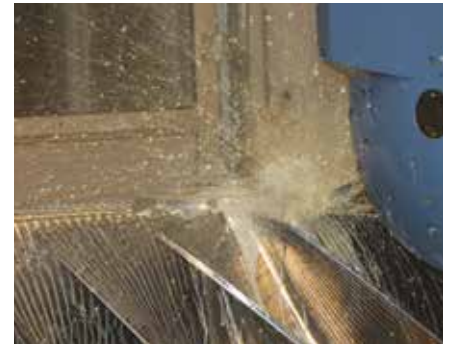
Inside the multi-skill machine: the milling process
