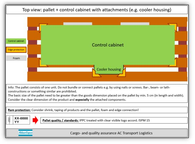
The pallets, EUR (EPAL) or disposable pallets in all dimensions must be 4-way capable and always have the characteristics according to ISPM 15.
