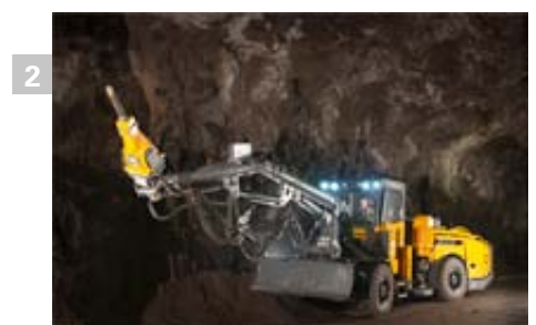
Scaletec for scaling
