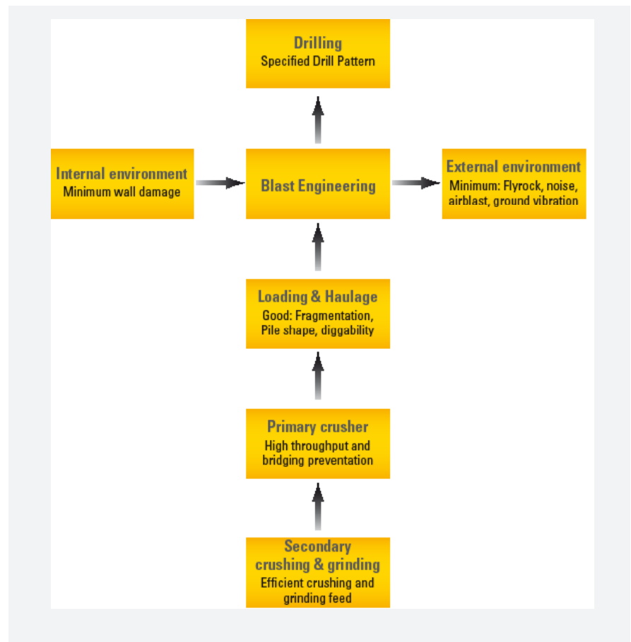
Figure 8. Simplified view of the five different stages of fragmentation, each with a different energy-product profile.
