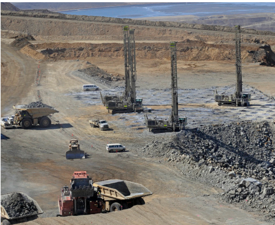
Photo: Blasthole drilling of 40ft (12m) benches at Newmont's Phoenix mine, Nevada, USA. See page 91.
