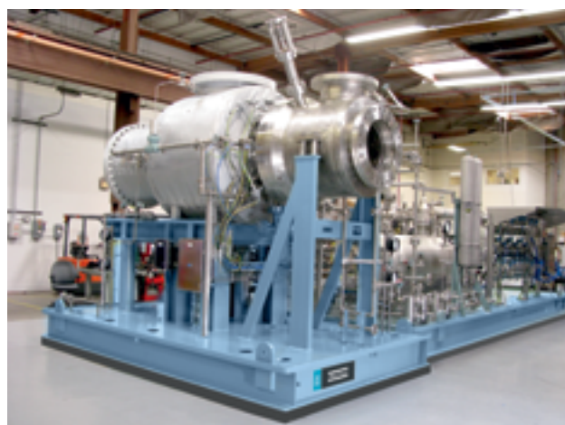
A turboexpander for cryogenic hydrocarbon separation.
