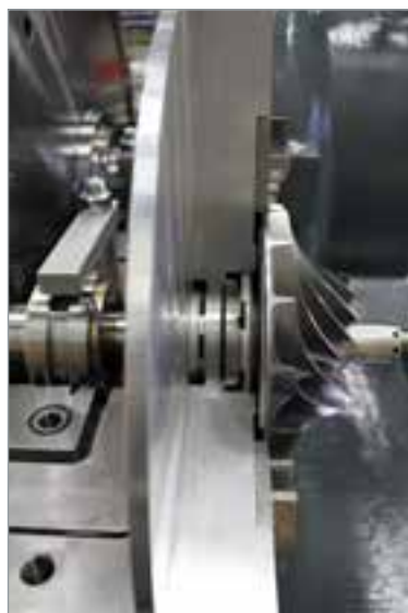
A dry face seal in deployment
