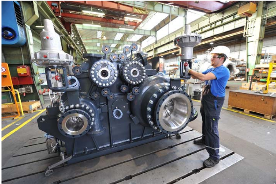
Figure 8: CO 2 -Compressor with eight stages – using dry face seals.
