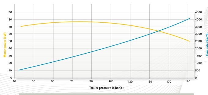
Average flow rate: 1590 Sm³/h\* considering reference conditions and correct installation as per Atlas Copco guidelines
