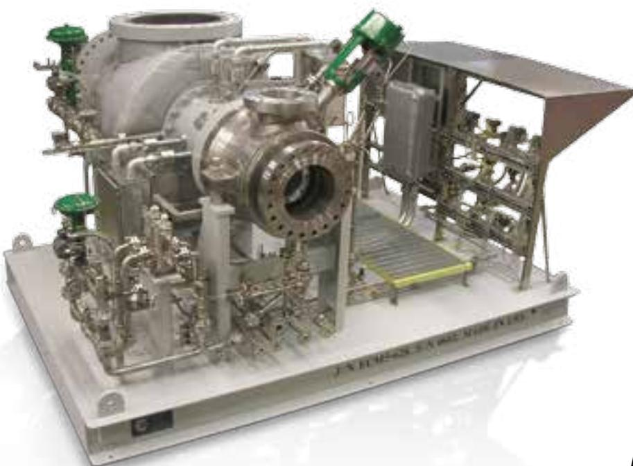
*Expander compressor with magnetic bearings for a gas-processing plant in Saudi Arabia*
