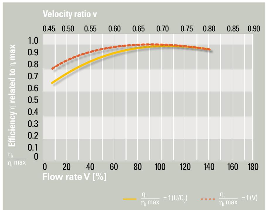
The typically flat turboexpander efficiency characteristic with various flow rates is illustrated here. Efficiency vs. the velocity ratio  $v$  (ratio tip speed to spouting velocity) is also shown.
