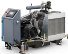
LB 40: Single-stage lubricated air and nitrogen booster for pressures up to 40 bar (580 psi).
