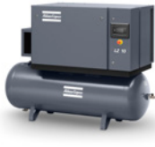
LZ: Elektronikon® Mk5 Touch controlled single-stage oil-free reciprocating compressor, silenced, with a maximum working pressure of 10 bar (145 psi).
