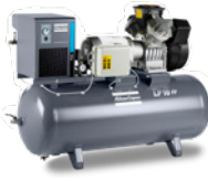
LF: Single-stage two-cylinder oil-free reciprocating compressor with a maximum working pressure of 10 bar (145 psi).
