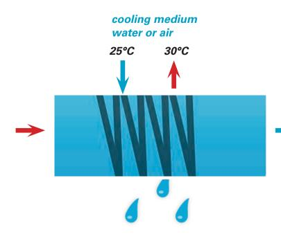
Cooling as drying method is very often used. Sometimes a heat exchanger with chilled cooling water is used to cool down the compressed air. At this low temperature, moisture is condensed into droplets of free water, which are collected and removed. This system is limited to the cooling water temperature and requires a water chiller to reduce the cooling water temperature.
