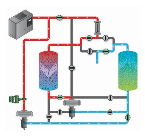
After heating, the desiccant beads need to cool down before they can start adsorbing again. The cooling can be done with dry compressed air, with cold ambient air or with cold compressed air. Each cooling method has his pros and cons.
