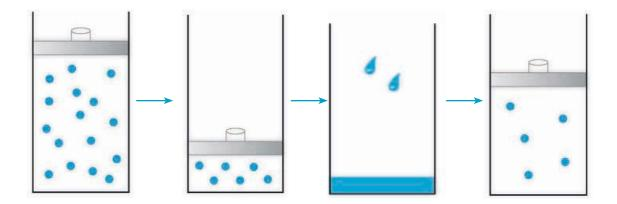
Absorption is an expensive method and the effluent of the dryer is a very aggressive liquid which needs to be treated as chemical waste. The absorption material needs to be continuously replaced with new material, this makes this system very expensive. The potential dew point suppression which can be achieved with this type of dryers is limited to 15°C.
