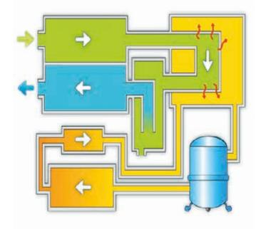
Adsorption dryers are mainly used when the required pressure dew point needs to be below 0°C. Most of those applications require dew points down to -40°C or even -70°C.
