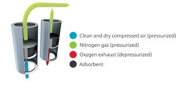
PSA technology isolates nitrogen molecules from other molecules in compressed air. Oxygen, CO2, water vapor and other gases are adsorbed. The result is virtually pure nitrogen at the outlet of the generator.
