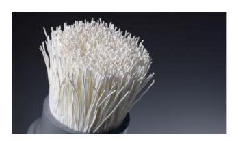
Membrane technology separates air into component gases by passing compressed air through semipermeable membranes consisting of bundles of individual hollow fibers.
