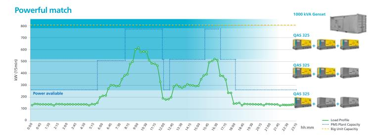
Note: this data is simulated. It's based on a typical industrial daily load diagram.
