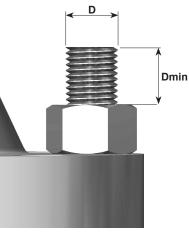
V-Series tensioners need a minimum of 1 x bolt diameter protruding above the hexagon or round nut.
