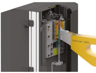
Gripper mechanism lowers to remove die from post
