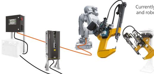
Currently only one SPR control panel and robot can be configured per die changer. In the future, the Atlas Copco SPR development team will be adding a software feature that will allow multiple robots to exchange dies on one die changer stand.
