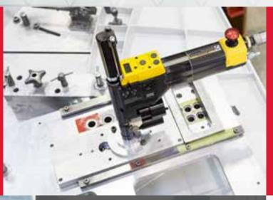
"BOGIE, STRUCTURE, RAILTRACK, WAGON PREPARATION" are the typical applications that need precise hole drilling. Automatic feeding from Atlas Copco Positive Feed Drills, PFD1100 and PFD1500, reduce the cycle time, prolong cutter life time and improves both productivity and quality. Drilling large holes in thick stacks is now a challenge in the past.
