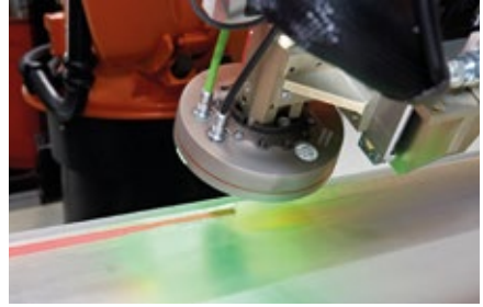
Example: Hem flange application with camera monitoring
