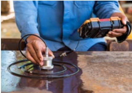
Ultrasonic test to detect imperfection or defect of steel plate
