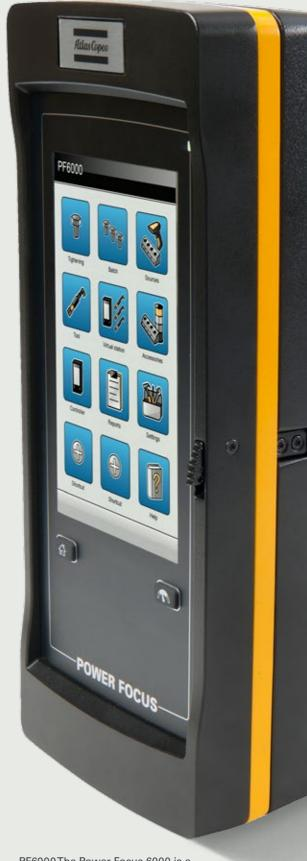
PF6000The Power Focus 6000 is a MultiTool Controller designed to optimize your assembly process.
