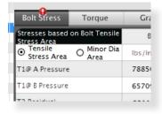
This tab also allows the user to switch between using bolt tensile stress area and bolt minor area to calculate bolt stress. When switching a new bolt load is calculated based on the type of bolt area chosen.
