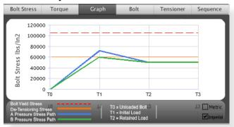
This tab displays the predicted bolt stress path over a 3 point time period.
