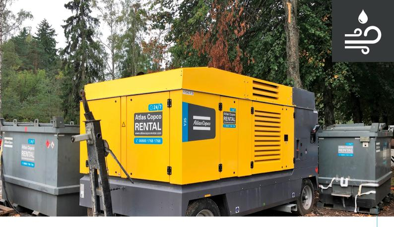
High-pressure compressor rented for geothermal well drilling to drill 7.2 kilometers of 500–600-meter deep wells. By using a DrillAir Y35 compressor, daily drilling depths could reach 500 meters.
