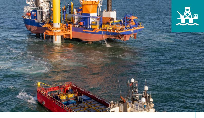
Oil-free compressed air for bubble curtains in the North Sea. Bubble curtains protect marine life against noise and vibrations during the build-up of wind turbines. 13 compressors type PTS1600+ delivered 100% oil-free air for the project.
