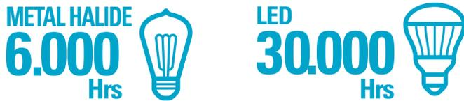
The tough conditions that light towers will experience in construction and mining applications make durability a key concern. One of the lesser known advantages of LED lighting is that it is less sensitive to temperature variations than many of its forebears. For example, hot and humid conditions do not affect the operation of LED in the same way they might affect a metal halide luminaire. Similarly, LEDs can operate fault-free in low temperatures too.
