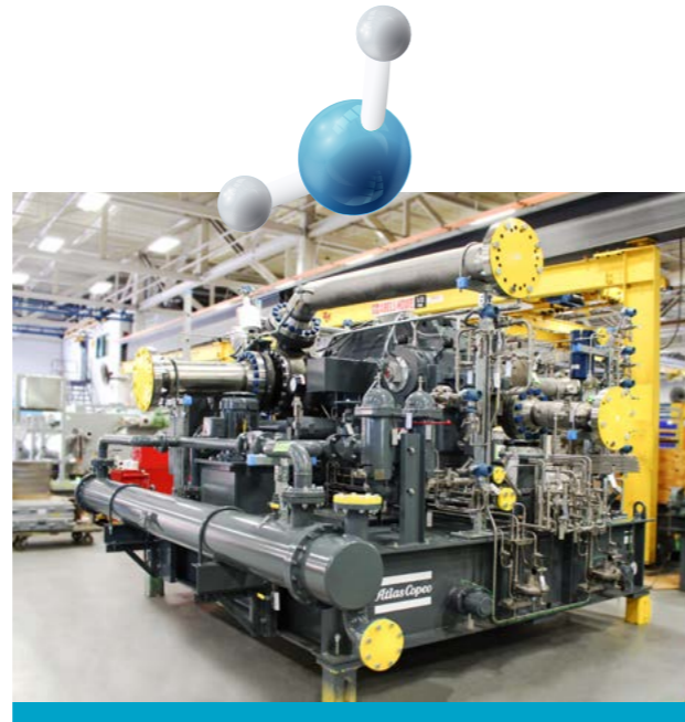
Integrally-g geared centrifugal compressor for oxy-combustion in sCO 2 power cycles.
