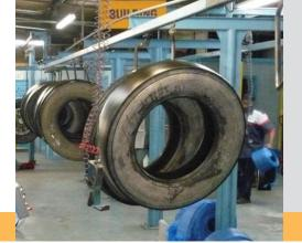
Using whichever method a customer prefers, new tread is placed on the prepared casing. The tires are then moved into a curing chamber where a high temperature, high pressure environment bonds the new tread securely to the tire casing.
