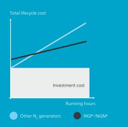
With an air factor\* of 1.8 (at 95%) to 5.5 (at 99.999%) and a special cycle time modulation algorithm, the running cost of the new NGP<sup>+</sup> can be reduced by 50%, compared to other  $N_2$  generators.
