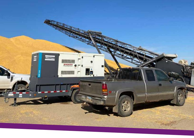
They called our partners at Interstate Power Systems— a leading distributor of high-quality power products for agriculture and other segments—to provide an outside power source to continue the harvest. Interstate Power Systems supplied Atlas Copco QAS 200, QAS 250 and QAS 330 generators to run the conveyors to unload corn and beans to outside storage.
