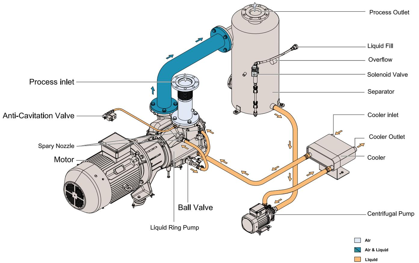
The LRP VSD+ series is the most energy efficient solution for applications with a high vapour load. The closed loop water circuit with integrated heat exchanger ensure the sealant water exiting the pump discharge is collected in the seal liquid reservoir and recirculated. The gained heat load is removed by passing through the stainless-steel heat exchanger contained within the LRP 700-1000 VSD+. All water level monitoring and top-up is a fully automated standard feature of the LRP VSD+.
