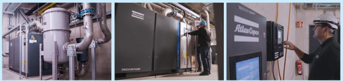
The Atlas Copco ES16 central controller can monitor and control multiple GHS VSD<sup>+</sup> vacuum pumps simultaneously. The smart control system balances and optimizes the performance of all machines, reducing the overall energy consumption.
