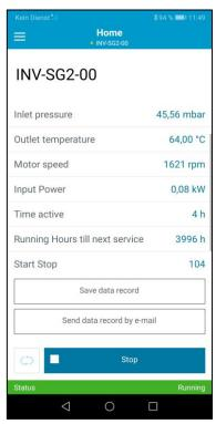
The app automatically connects via an integrated Bluetooth interface as soon as the pump is started.
