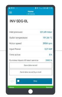
With the VSD<sup>+</sup> app, you also have live visualizations of the actual performance and settings. You can monitor details such as inlet pressure, rotor speed, running hours and service intervals.
