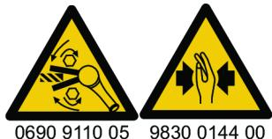
Check the rotational direction of the tool before start! A start in an unexpected rotational direction can cause bodily injury or property damage. Moving parts can crush and cut.
