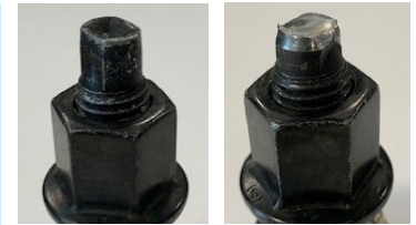
These photos show an unused and a broken Two Flat screw tip
